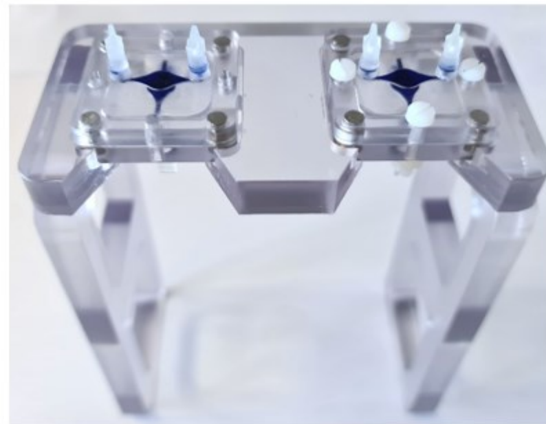
SoC devices placed in dedicated support
