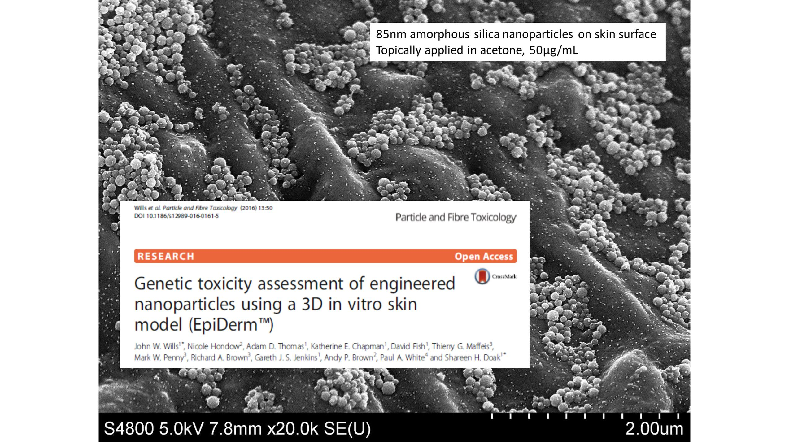
Scanning electron micrograph (SEM) showing a dense distribution of small, spherical, amorphous silica nanoparticles on a textured skin surface. The nanoparticles are approximately 85 nm in diameter and are clustered together, covering the surface irregularities. The background shows the complex, undulating topography of the skin surface.
